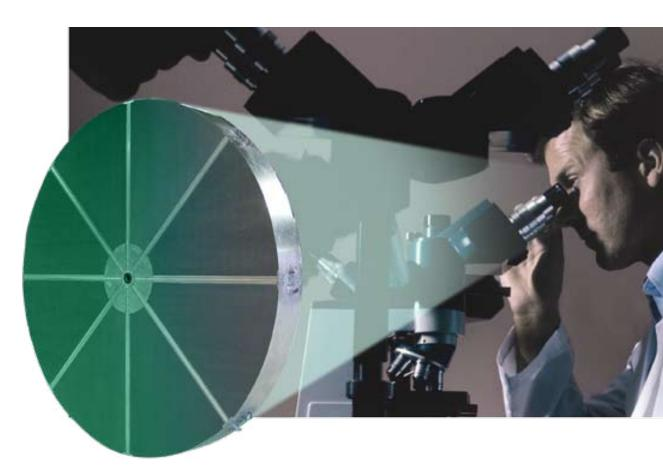
The PPM molecular sieve rotor is intended for use in dehumidifier applications where entering air is dry and/or hot, and where the processed dry air must be even dryer. Examples of such applications are plastic hopper dryers requiring dew points below -40 °C (-40 °F), and production rooms for lithium-ion batteries requiring a dew point of -60 °C (-76 °F) or lower.
